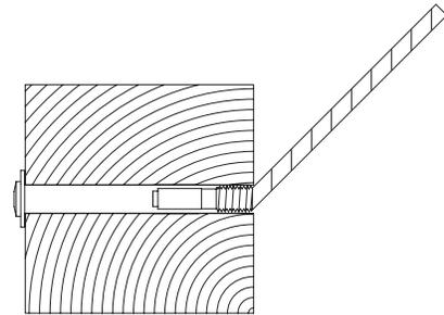
**d) Hardware used for stairs or severe slopes.** You can use any of the fittings with a fork or an eye in conjunction with a Lag Eye, to accommodate stairs and slopes. These fittings are Adjust-A-Jaw® and Adjust-A-Body® with Threaded Eye tensioners, and Ultra-tec® Fixed Jaw and Push-Lock™ with threaded eye non-tensioning fittings.
