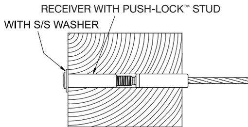
Note: With the Invisiware® Receiver or Receiver with Push-Lock™ stud tensioner, you will need up to 3-3/4" of space between the back of your end post and any structure to insert the fitting into the end post from the back side.
