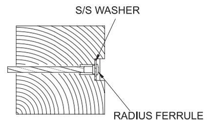
Note: With the Radius Ferrule, Push-Lock™ or Pull-Lock™ fittings, you will need approximately 2-1/2" of space between the back of your end post and any structure to insert the fitting into the end post from the back side.
