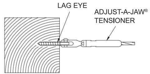
The other end of each cable run can be either a tensioner (above) or a non-tensioning device. Following are **non-tensioning devices**.
