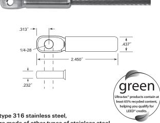
Push-Lock™ fittings are made of type 316 stainless steel, with the exception of internal components that are made of other types of stainless steel.
